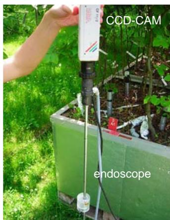
Endoscope and CCD-camera
