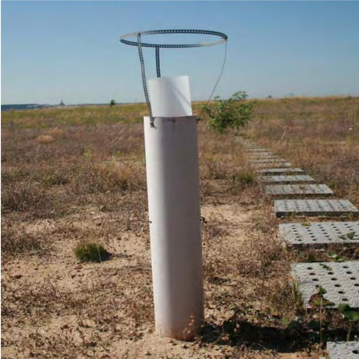
Fig. 3.1: Bulk deposition sampler.
