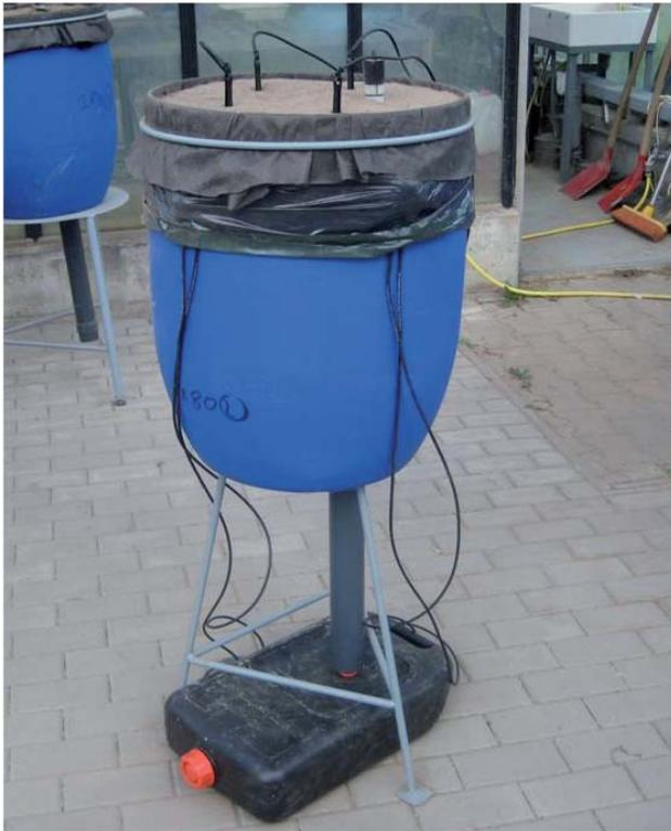
Figure 1: Modified wick lysimeter and drip irrigation system
