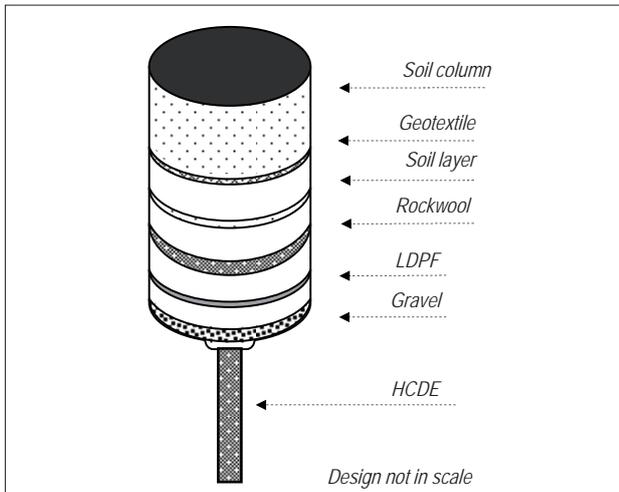
Figure 2: Schematic diagram of the lysimeter
