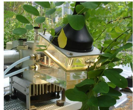
Fig. 3: Climatic controlled mini-cuvette chamber for measuring CO<sub>2</sub> and H<sub>2</sub>O exchange of leaves.
