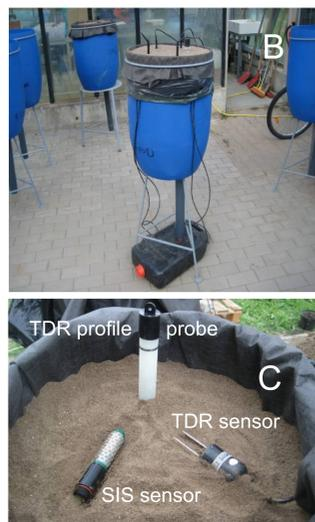
Fig. 2: (A) Schematic diagram of the new wick lysimeter, (B) lysimeter (C) installed TDR systems and SIS Smart-Irrigation-Sensor for the monitoring of soil water content and soil matrix potential.
